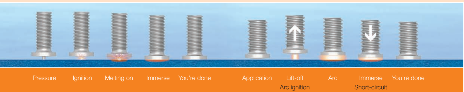
Capacitor discharge stud welding with tip ignition (contact welding)
